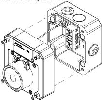
Once the screws are removed the cover will hang down out of the way to gain access to the Ex e terminal block, the internal earth terminal and mounting hole recesses.
